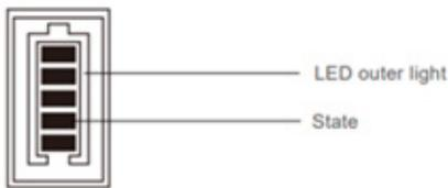
Figure 5: LED indicator lights on Giter and rocker switch
